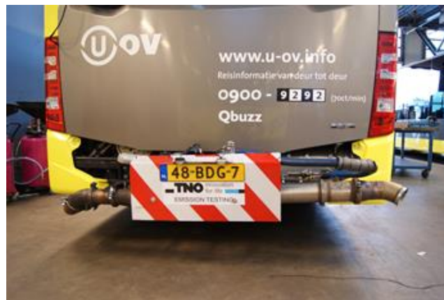
Figure 2: PEMS installed on the exhaust of the Mercedes Citaro.
